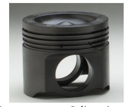
Heavy-duty piston designs have evolved over the past many years as a result of increasing cylinder pressure specifications. Early model engine pistons were predominantly one piece aluminum designs, which later evolved into two piece articulated designs with steel crowns and aluminum skirts. Ever increasing cylinder pressures led to 1 piece steel pistons, and eventually to more recent friction welded designs.
